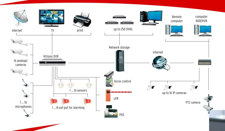
KVision DVR is a modern surveillance technology for digital video and audio recordings, capable of data storing and processing, as well as of creating long-term available databases.
